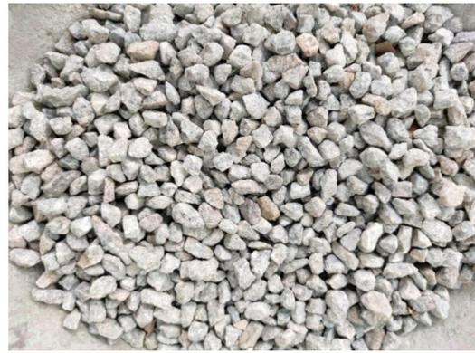
Figure 6: Coarse aggregates
